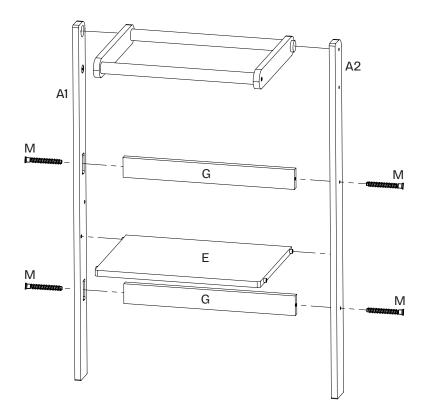
USE SCREWS "M", ALLEN KEY "K" AND SCREW PARTS "A1" AND "A2" WITH PARTS "G" AND PART "E" AS SHOWN.
