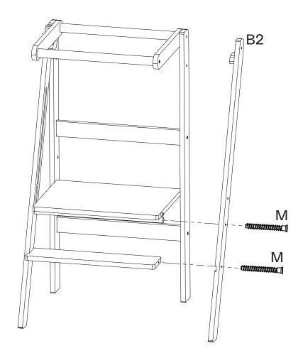
USE SCREWS "M", ALLEN KEY "K" AND SCREW PART "B2" AS SHOWN.
