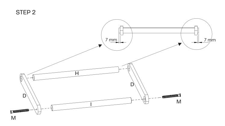
TAKE SCREWS "M", ALLEN KEY "K" AND SCREW x2 PARTS "D" WITH PART "H" AND PART "I" AS SHOWN.
