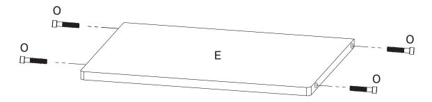
TAKE SCREWS "O" AND ALLEN KEY "L" AND SCREW ALL SCREWS FULLY IN.
